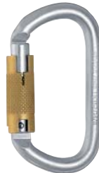
K4241Z007 STEEL OVAL CONNECTOR TRIPLE LOCK with key lock and triplelock gate Weight: 195 g Strength: ◀▶ 30 kN, ◀ 9 kN, ◀ 8 kN unique number CE 1015, EN 362
