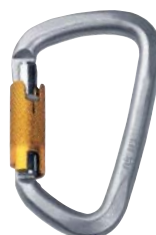
K4081ZO D STEEL CONNECTOR TRIPLE LOCK with triple lock gate, key lock, zinc plated ◀▶ 50 kN ◀ 13 kN ◀ 20 kN gate opening (d) 25 mm ■ 267 g ■ 9,42 oz. unique number CE 1015 ■ EN 362
