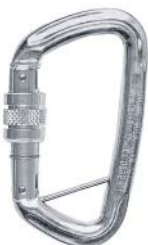
K4280PP D BAR CARABINER SCREW GATE with screw gate and captive bar, polished ◀▶ 30 kN ◀ 9 kN ◀ 11 kN gate opening (d) 19 mm ■ 76 g CE 0639 ■ EN 362 ■ EN 12275
