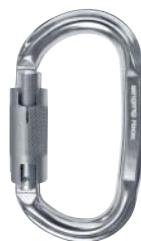
K4640PP CARABINER LOCK OVAL TWL with twist lock, polished ◀▶ 24 kN ◀ 8 kN ◀ 7 kN gate opening (d) 19 mm ■ 80 g CE 0639 ■ EN 362
