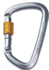
K4080ZO D STEEL CONNECTOR SCREW with screw gate, key lock, zinc plated ◀▶ 50 kN ◀ 13 kN ◀ 20 kN gate opening (d) 25 mm ■ 255 g ■ 9 oz. unique number CE 1015 ■ EN 362
