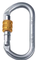
K4241Z005 OVAL STEEL CONNECTOR SCREW with screw gate, key lock ◀▶ 30 kN ◀ 9 kN ◀ 8 kN gate opening (d) 17 mm zinc-plated ■ 176 g ■ 6,21 oz unique number CE 1015 ■ EN 362
